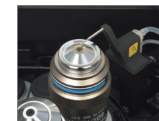
Dual micro nozzle keeps the proper amount of water on the tip of objectives.
