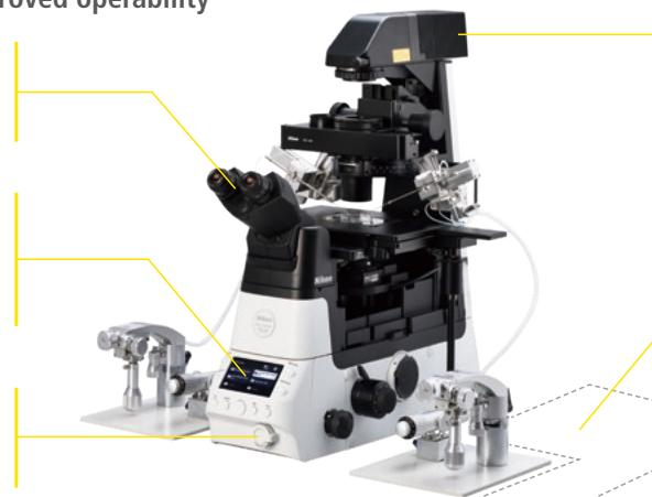
Long-life LED illumination provides bright images even during high-magnification observation. Recording and automatic reproduction of adjusted brightnesses has also been achieved.
