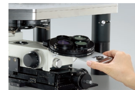
The condenser and polarizer turret can be simply and quickly removed.
