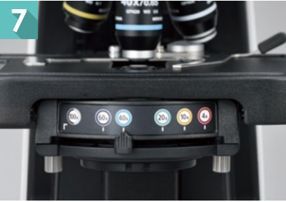
The best aperture can be set intuitively The lever positions of the condenser aperture are color-coded and matching the objectives.
