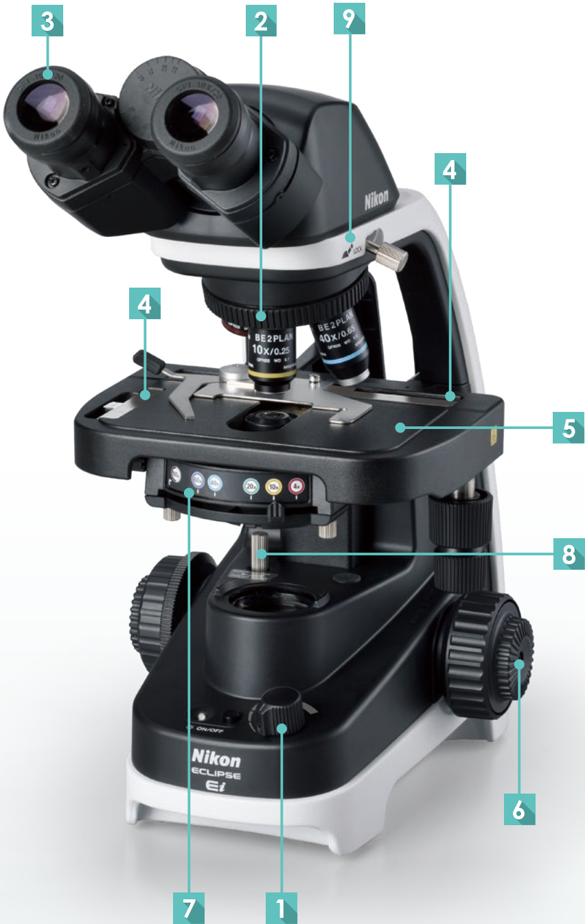
Illustrative presentation of handles The handles for moving the stage in the X/Y direction are displayed using illustrations of their respective shapes.
