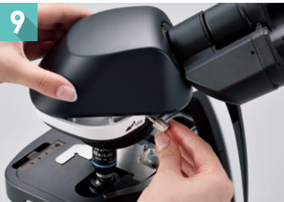
Tube orientation displayed during storage The tube can be rotated to reduce the space required for storage by loosening the tube locking screw. The tube is designed so that it does not fall.
