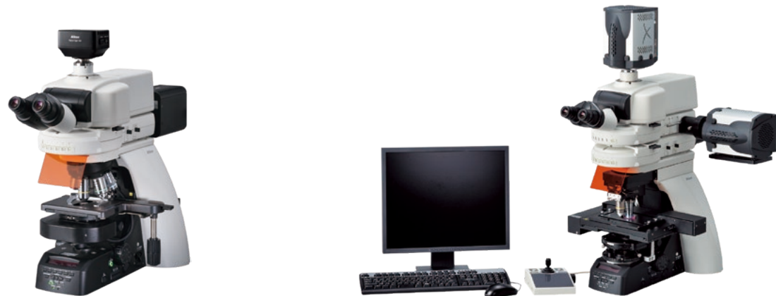
Ni-E (Focusing stage) configured with motorized epi-fluorescence illuminator, motorized condenser and motorized quadrocular tilting tube and the Digital Sight 100 camera
