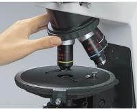
lengths and longer working distances provide more working space around the nosepiece.
