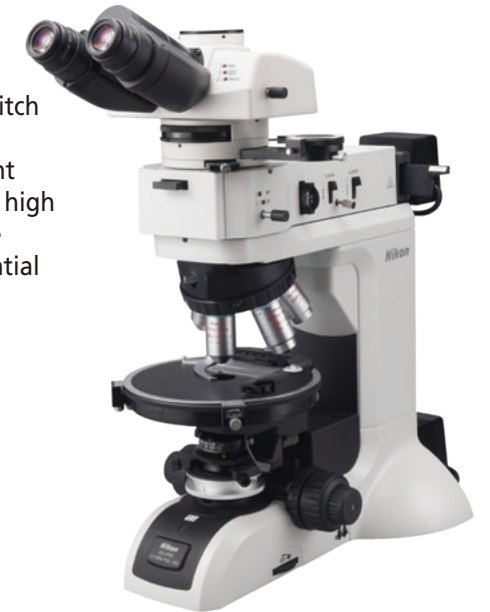
ECLIPSE LV100N POL LED (Diascopic/Episcopic illumination type)
