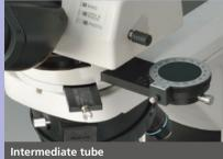
The intermediate tube incorporates a Bertrand lens as standard, enabling both the observation and capture of conoscopic and orthoscopic images. The Bertrand lens is focusable and centerable. The high precision slider-type analyzer can be rotated a full 360° with a precision vernier scale. A P-LC tint plate slider with full and quarter
