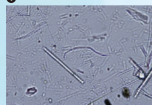
Chrysotile and amosite (refraction index of the liquid nD = 1.605, CFI P Achromat 40x)
