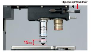
Objective retraction mechanism
