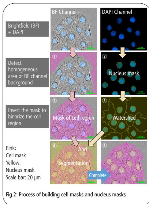
Fig.2: Process of building cell masks and nucleus masks
