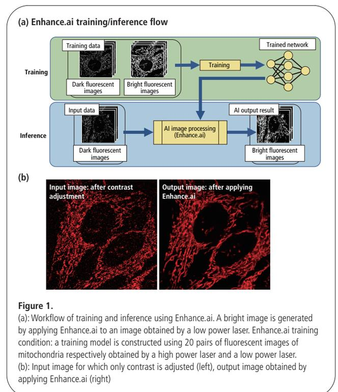
**Figure 1.** (a): Workflow of training and inference using Enhance.ai. A bright image is generated by applying Enhance.ai to an image obtained by a low power laser. Enhance.ai training condition: a training model is constructed using 20 pairs of fluorescent images of mitochondria respectively obtained by a high power laser and a low power laser. (b): Input image for which only contrast is adjusted (left), output image obtained by applying Enhance.ai (right)
