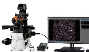
The High Content Analysis (HCA) option of NIS-Elements imaging software is installed in the Ti2-E microscope and camera combination. Quick and easy execution, from image acquisition to analysis, is possible with one system.
