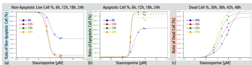
Fig. 13: Staurosporine dose-response curve and  $\text{EC}_{50}$  value at each drug treatment time
